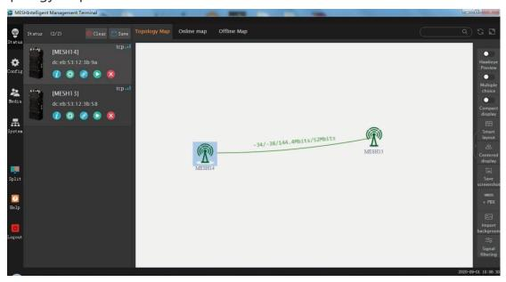
The topology map shows the link connection status between devices. The icons are divided into three states: intelligent network, base station, and client. The link has three colors of green, yellow and red to indicate the quality of signal strength. Double-click the device icon to display the detailed information of the device.
