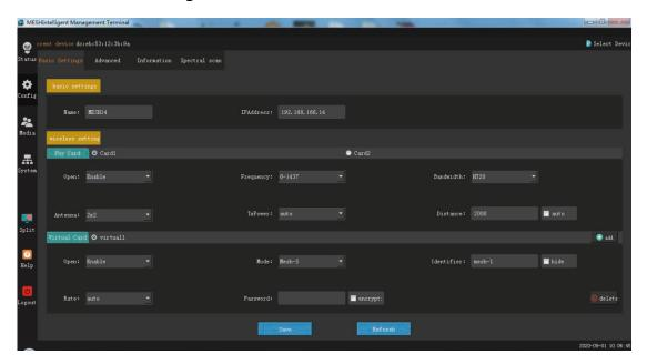
Basic settings can set equipment IP, wireless and other information, one-key configuration is convenient and quick, among which the smart network mode, only need to configure the frequency, bandwidth, distance, identification code these parameters, the smart network ensures that these parameters are consistent. It can be connected normally, and the distance needs to be slightly larger than the actual distance (m)
