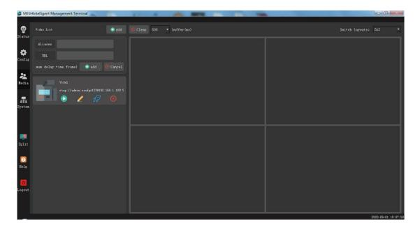
Media management can play all network media, including http, rtsp, udp, rtmp, rtp, mms and other streaming media, and supports up to 4x4 (16 channels) simultaneous playback.
